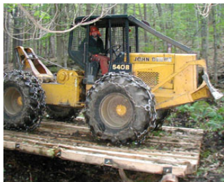
Conservation Districts rent Portable Skidder Bridges to help protect waterways during logging operations.
